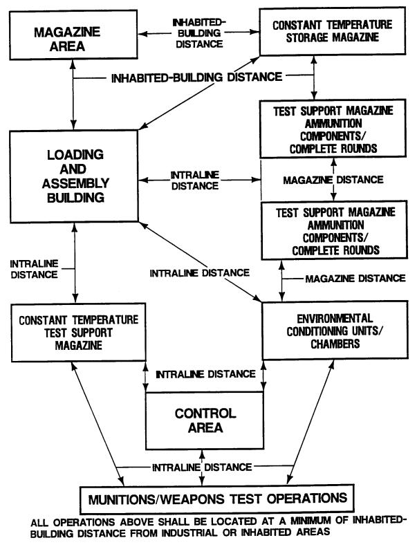
Figure 22-1. Layout - Munitions/weapons test operations.
