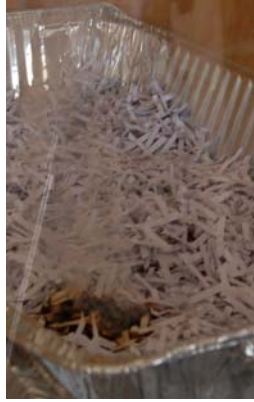
Figure 9 Picture taken 10 minutes after completion of the experiments. Self-sustaining smoldering ignition is observed in the shredded paper bed at 5 % moisture content (dry basis). This image was taken for a 6 mm screen installed behind the vent. The obscuration in the image was due to smoke production due to smoldering combustion.
