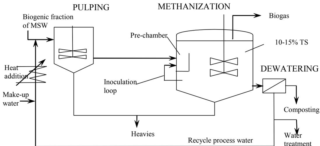
**Fig. H-11. Schematic of Single-Stage Low Solids Anaerobic Digestion System (Waasa, Finland)**
