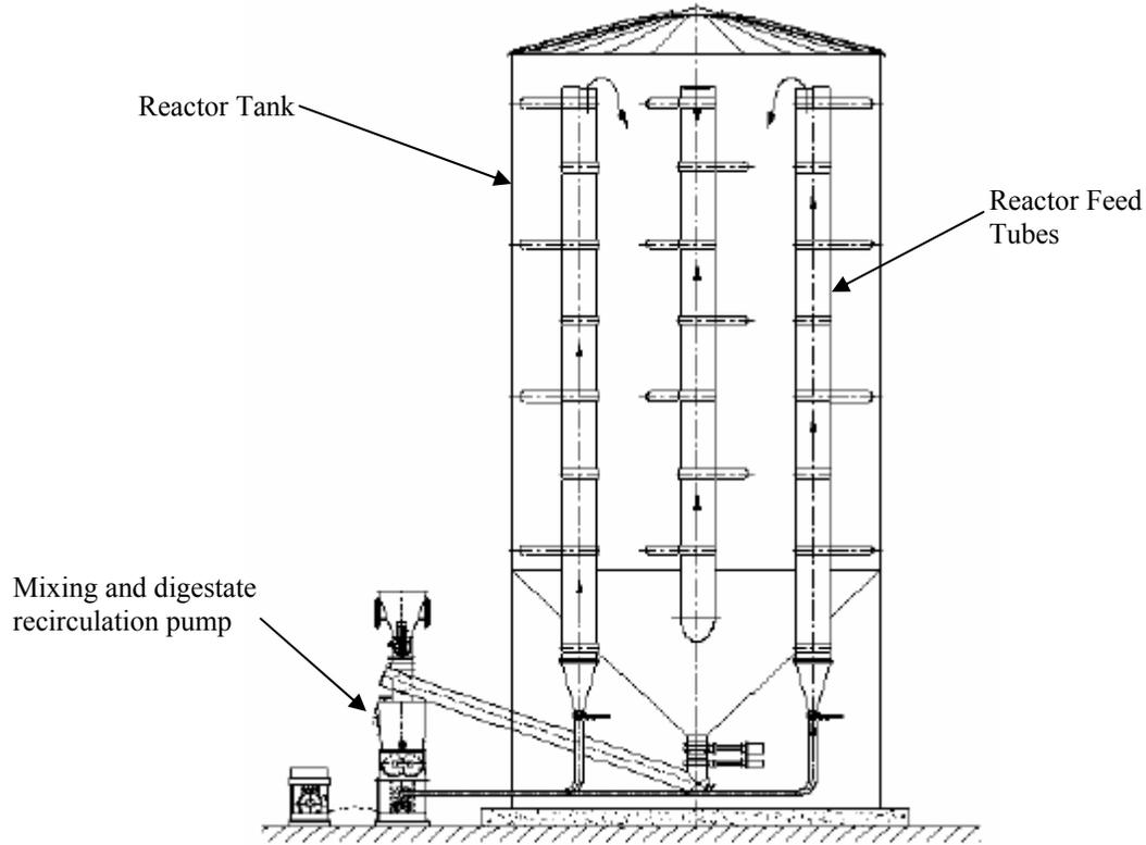
**Fig. H-15. Drawing of the DRANCO reactor (source OWS)**
