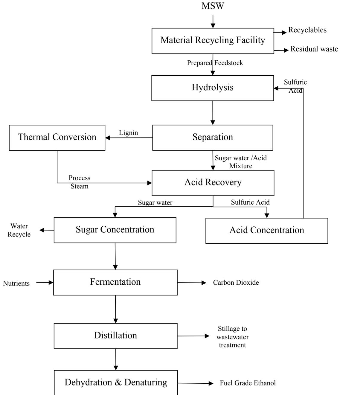
**Fig. H-1 Masada Oxynol Process Flow Diagram (Masada Resource Group)**
