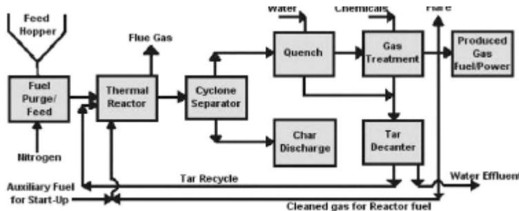
Fig. F-14. WGT Process Schematic.<sup>288</sup>
