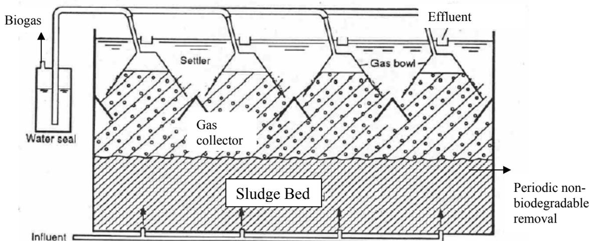
**Fig. H-6. Schematic of a UASB Bioreactor<sup>300</sup>**
