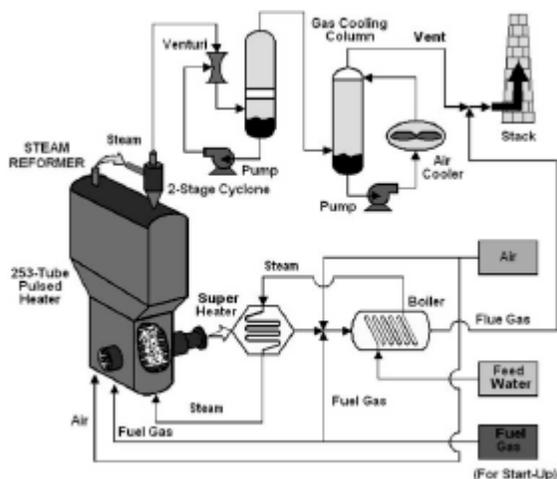
Fig. F-12. Schematic of the MTCI PulseEnhanced Steam Reformer Technology.<sup>280</sup>
