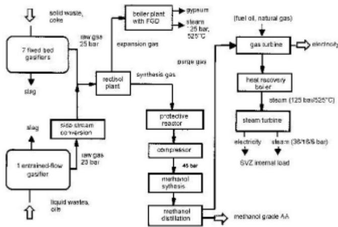
Fig. F-1. Schematic of the SVZ Waste Utilization Concept in Polygeneration Configuration.<sup>126</sup>
