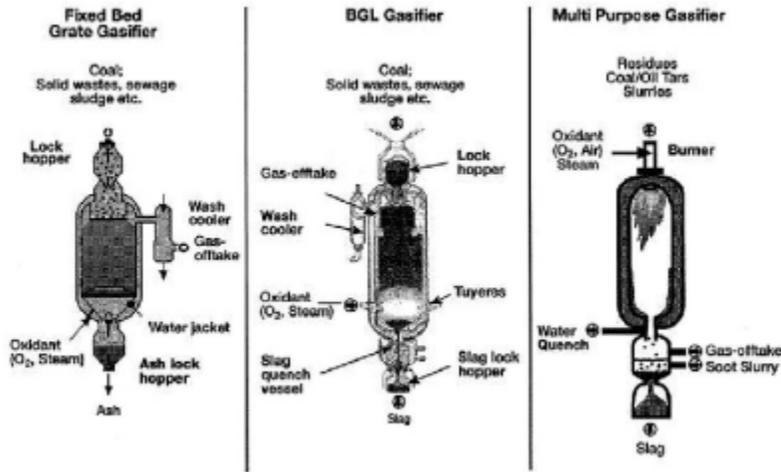
Fig. F-2. Type of Gasifiers Used at the SVZ Installation.<sup>127</sup>
