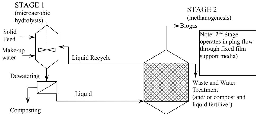
**Fig. H-10. Simple Schematic of Biopercolat Process (high solids 1<sup>st</sup> stage, low solids 2<sup>nd</sup> stage)**
