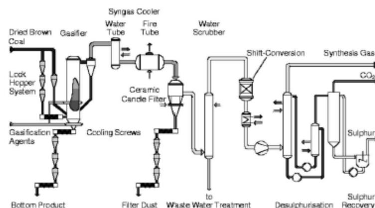
Fig. F-6. Flow Diagram of the HTW Demonstration Plant.<sup>182,183</sup>
