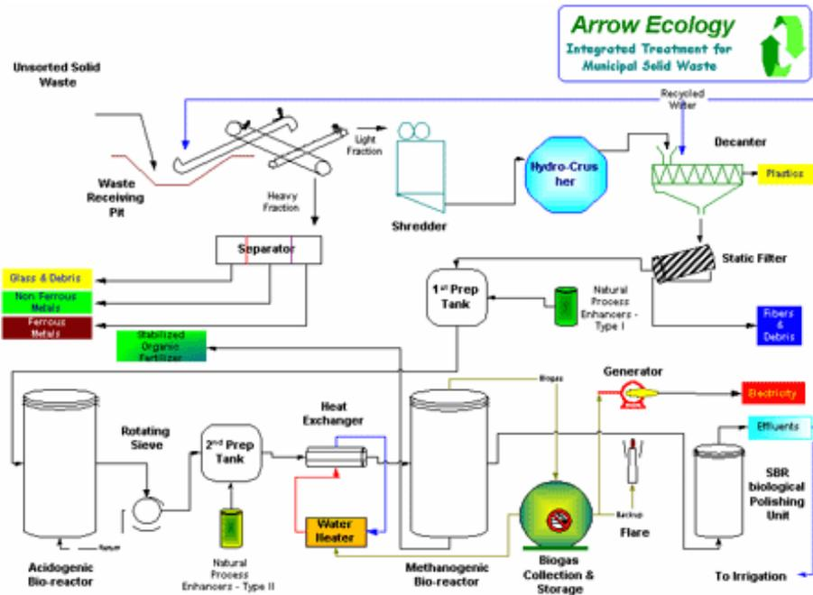
Fig. H-5. Schematic of the ArrowBio Process<sup>299</sup>
