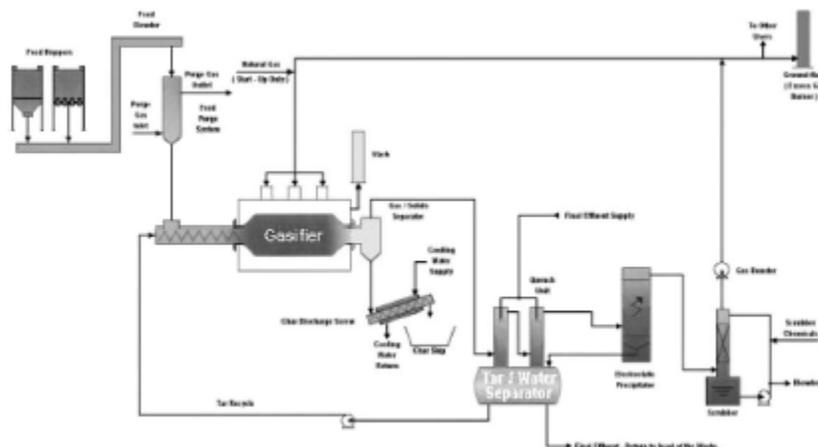
**Fig. F-15. Schematic of a WGT Demonstration Plant.**<sup>289</sup>
