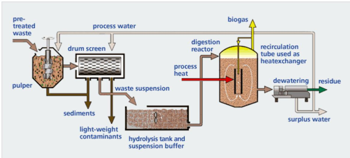
Fig. H-12. Linde-KCA two stage wet digestion system (source Linde-KCA)
