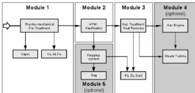
Fig. F-5. Schematic Concept of the Krupp Uhde PreCon Process.<sup>180,181</sup>
