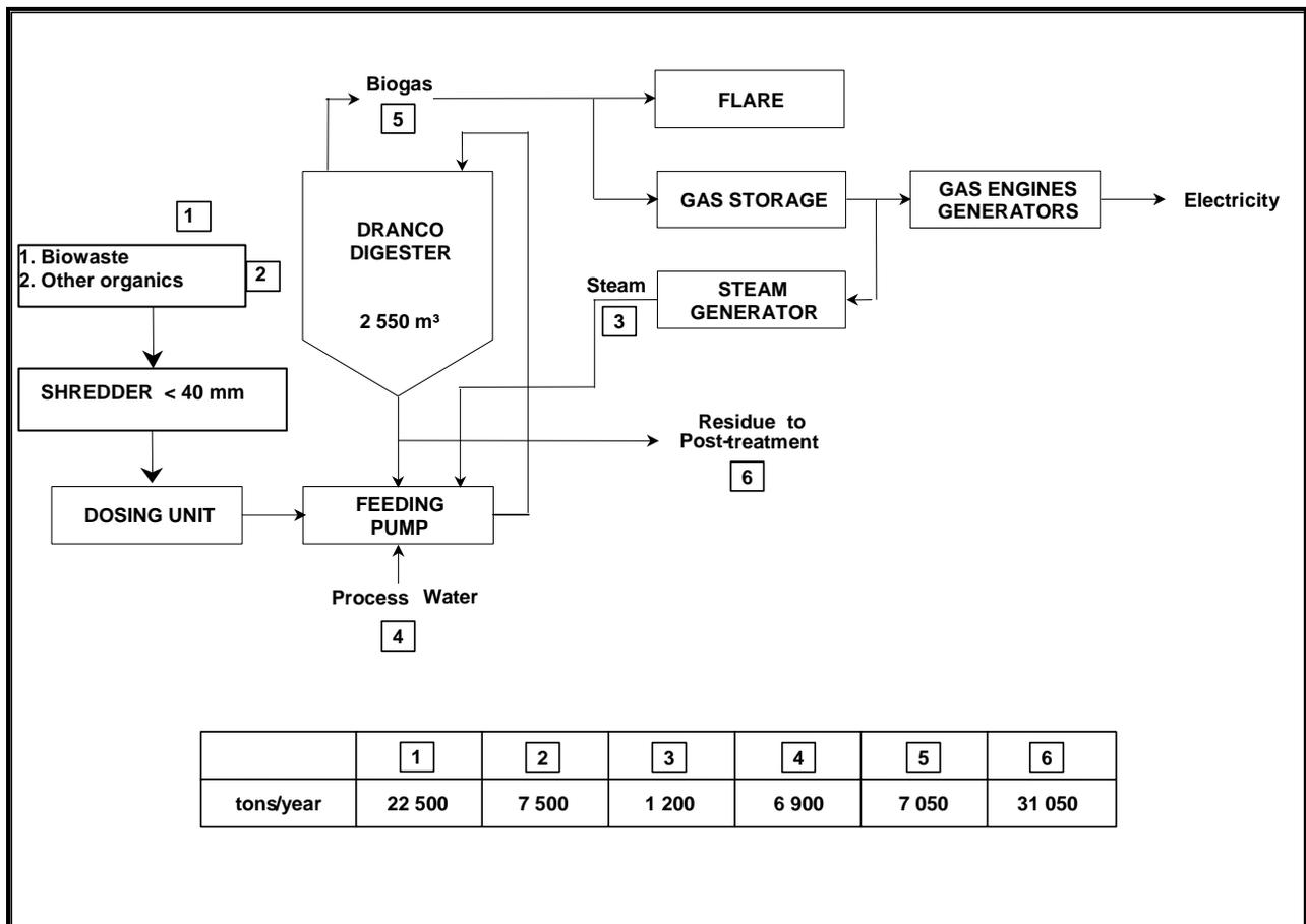
Fig. H-14. Schematic and mass balance of the DRANCO process (source: OWS)
