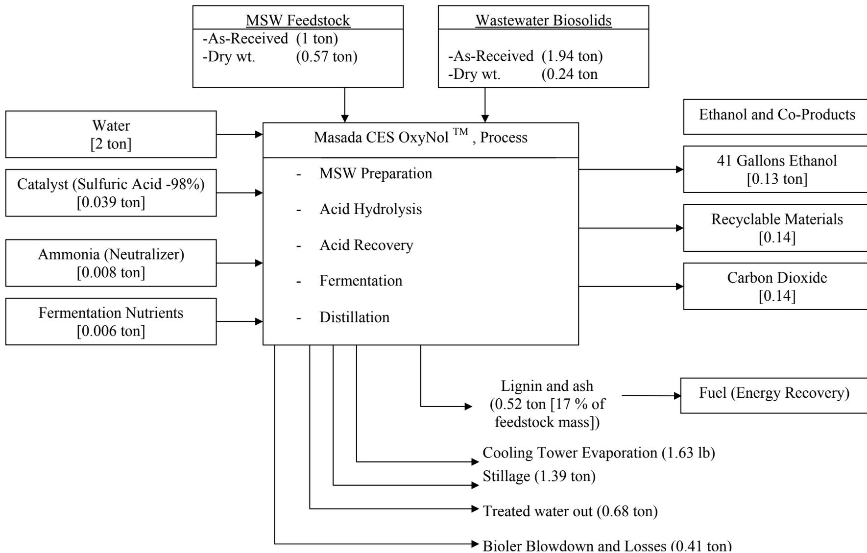
Fig. H-2. Masada Process Material Balance for 1 ton MSW and 1.94 ton Biosolids Input
