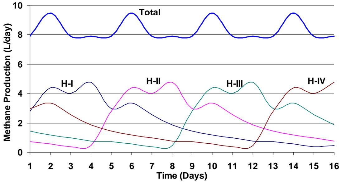
Fig. H-8. Simulated Biogas Production Rate for Lab-Scale APS Digester System
