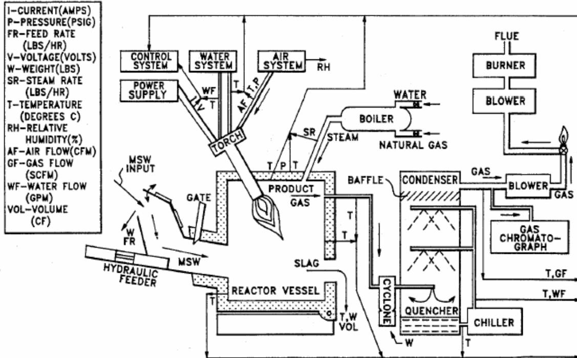
Fig. G-1. Schematic of RCL Research Plasma Gasifier. (adapted from US patent 5280757)
