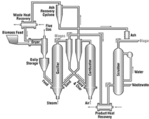
Fig. F-8. Schematic of the BCL/FERCO Allothermal CFB Gasification Process.<sup>247</sup>
