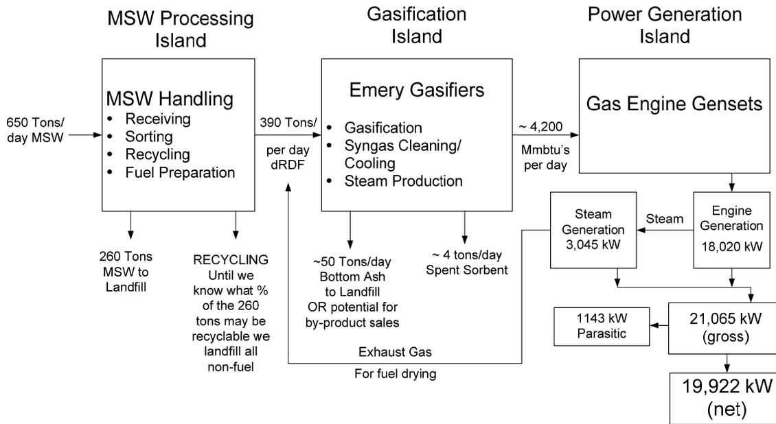
**Fig. F-3. Process Flow Diagram for 20 MWe MSW Gasification Power Plant recently proposed to a municipality in California**
