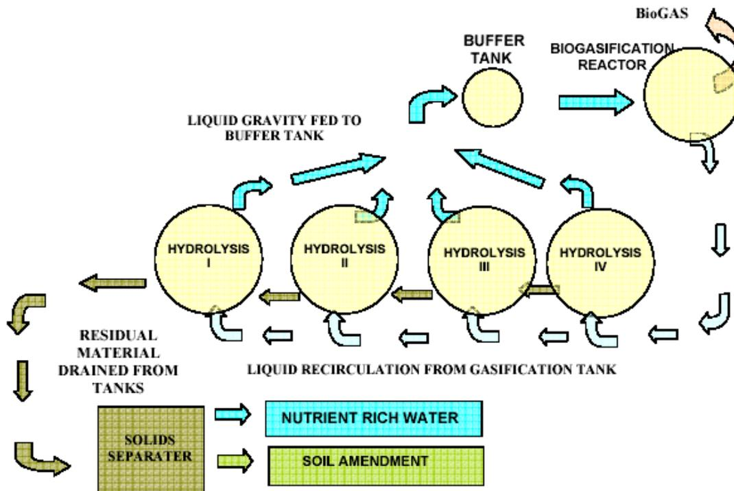
Fig. H-7. Schematic of APS Digester System Showing 4 Hydrolysis Vessels (Courtesy R. Zhang)
