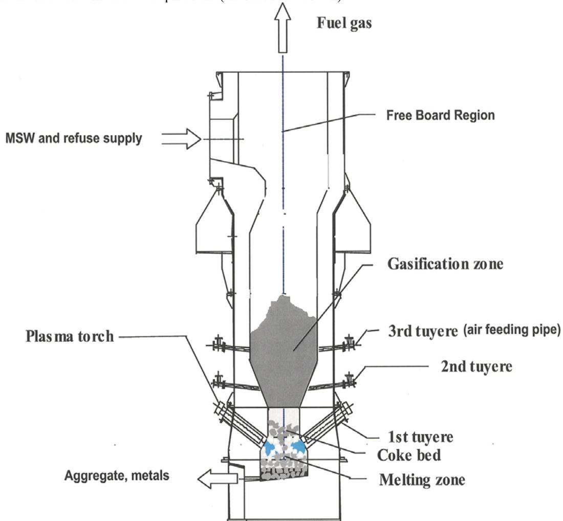
**Fig. G-4 Conceptual Cross-Section of Westinghouse Plasma Corporation Plasma Direct Melting Reactor (tuyere is blast furnace terminology for air injection port)**
