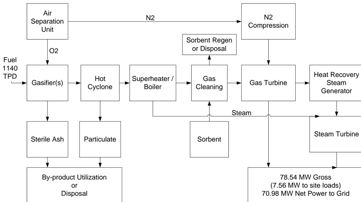
**Fig.F 4. Simplified Process Flow Diagram for 70 MWe Biomass Gasification Power Plant (DESIGNED UNDER U.S. DOE Contract DE-FC26-01NT41531)**
