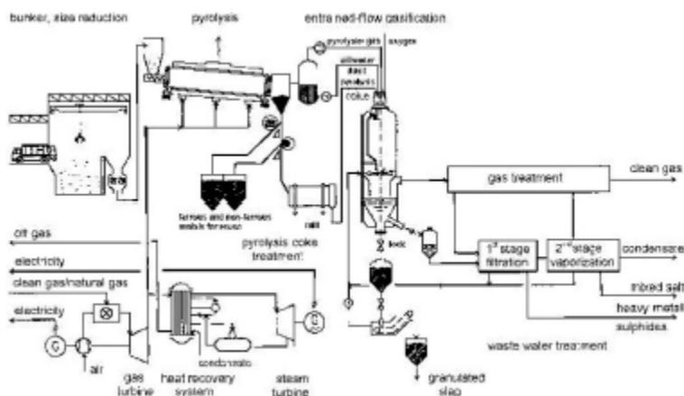
Fig. F-8. Scheme of the Noell-KRC Conversion Process.<sup>219</sup>
