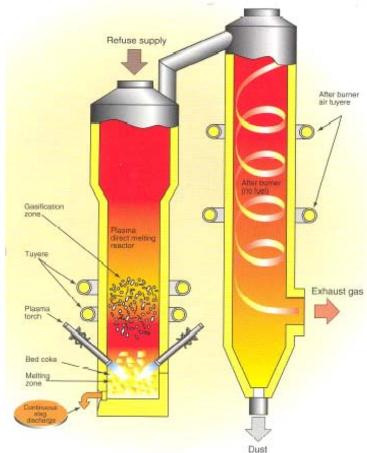
**Figure G-3 Schematic of Hitachi Metals plasma assisted gasifier and gas burner**
