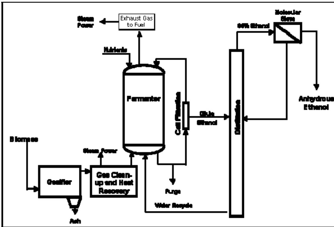
**Fig. H-9 Schematic of BRI gasification and fermentation of ethanol process (Source: BRI)**
