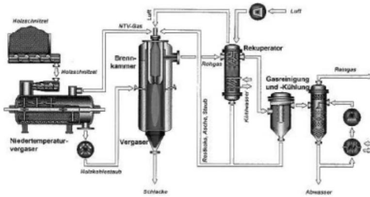
Fig. F-13. Schematic of the Carbo-V-Gasification Process.<sup>282</sup>
