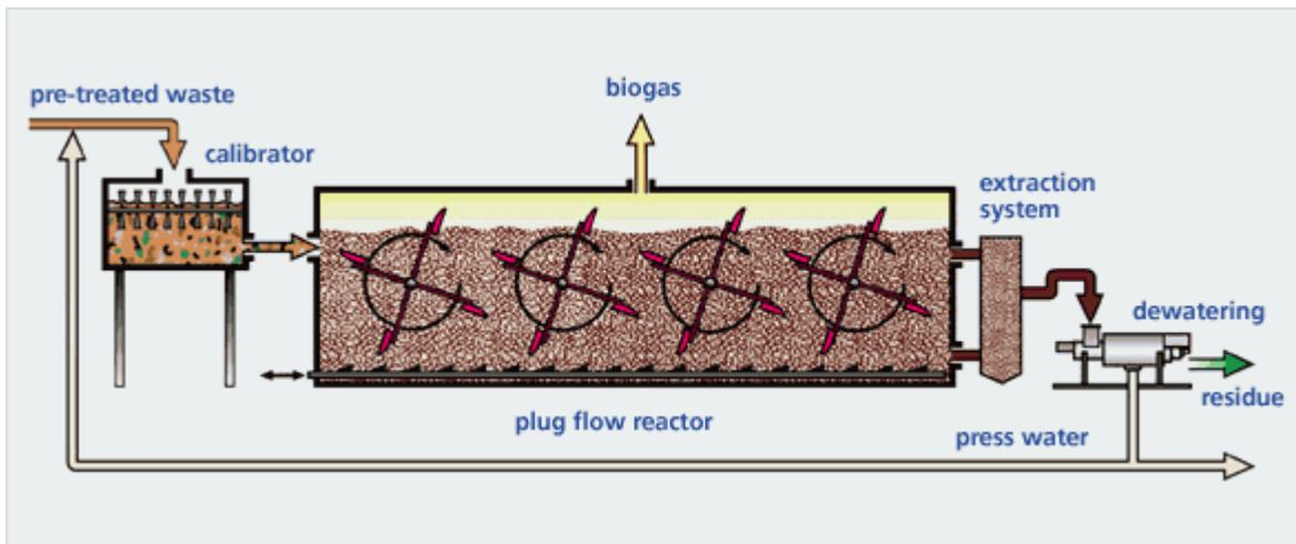
Fig. H-13. Linde-KCA dry digestion plug flow system (source: Linde-KCA)
