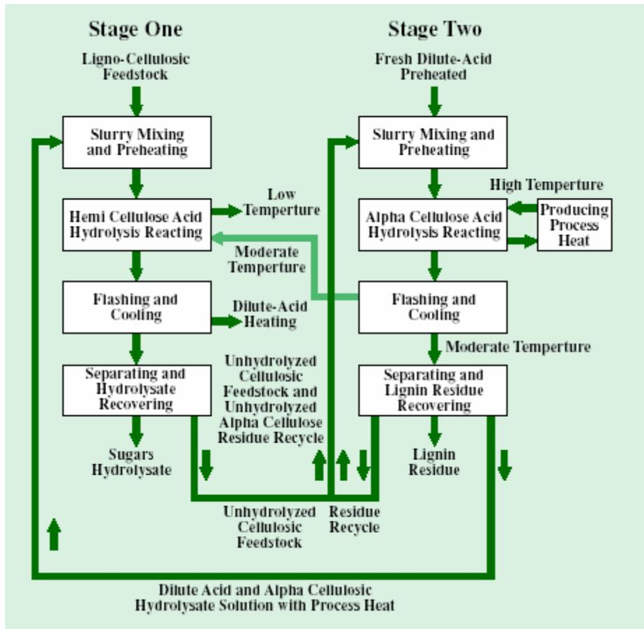
Fig. H-4 BEI/Genahol Hydrolysis and Ethanol Process Schematic
