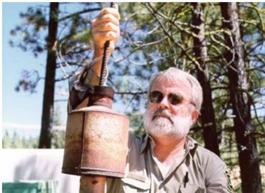
Photograph 4-9. Spark Arrester being Checked for Internal Burn Out or Modification
