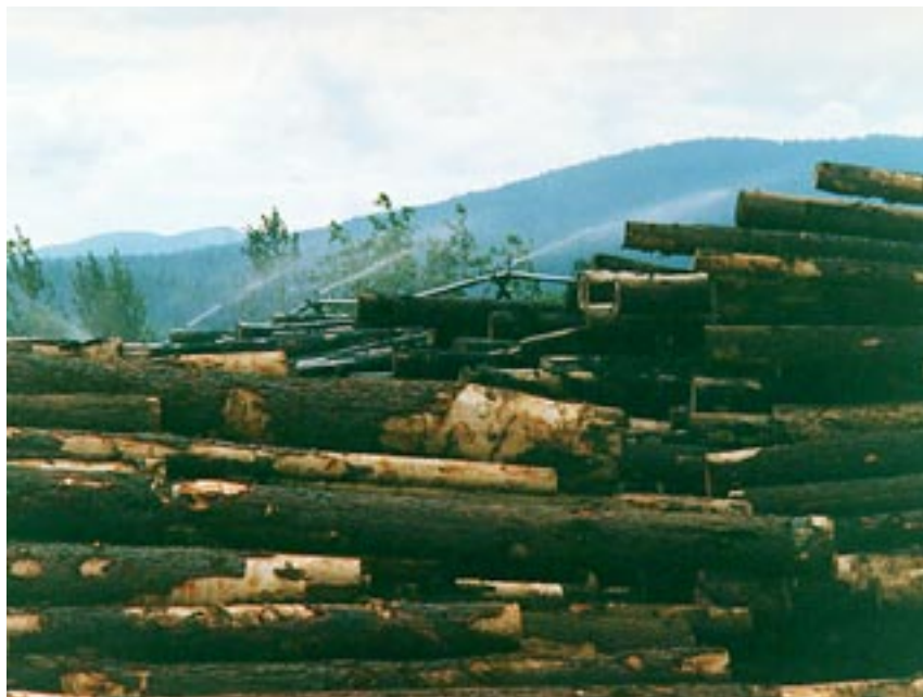
Photograph 13-4. Sprinklered Log Deck
