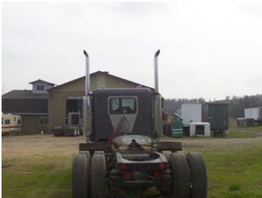
Photograph 7-4. Exhaust Stack on Semi-Truck with 90-Degree Bend and Shield
