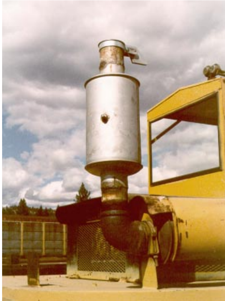
Photograph 4-7. Retention Spark Arrester, Plug Type
