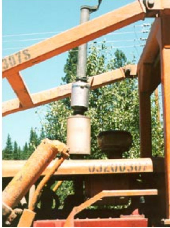
Photograph 4-5. Retention Spark Arrester (Top)
