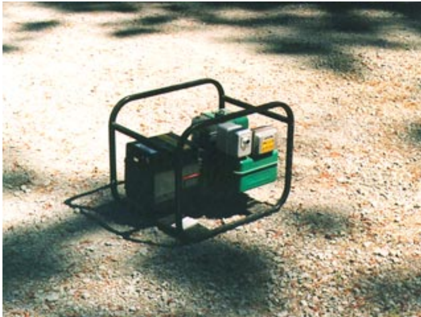
Photograph 5-4. Generator with Spark Arrester and Clearance
