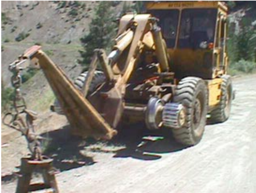
Photograph 7-7. Rail Placement Device
