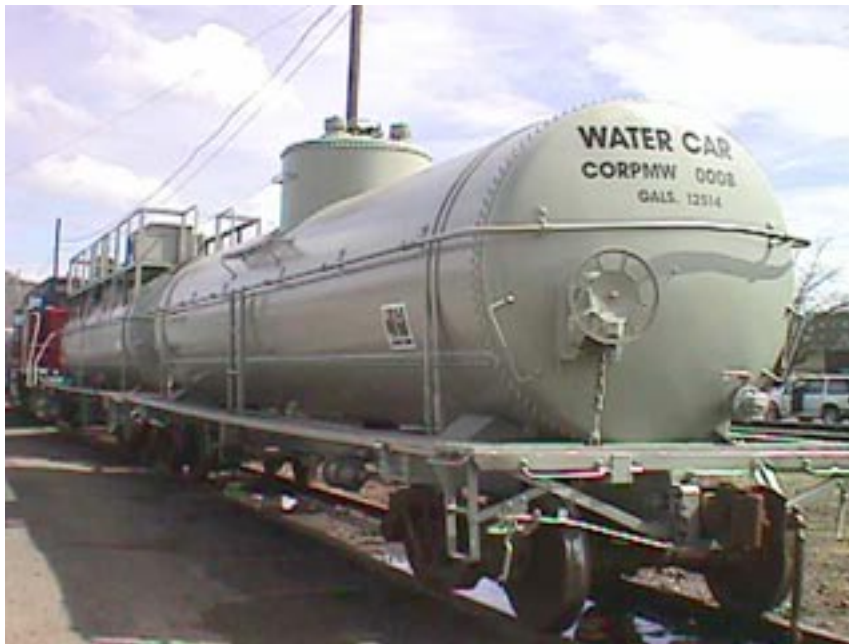
Photograph 8-3. Water Car with Spray Bars
