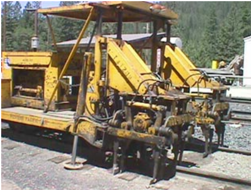
Photograph 7-8. Tie Replacement Equipment
