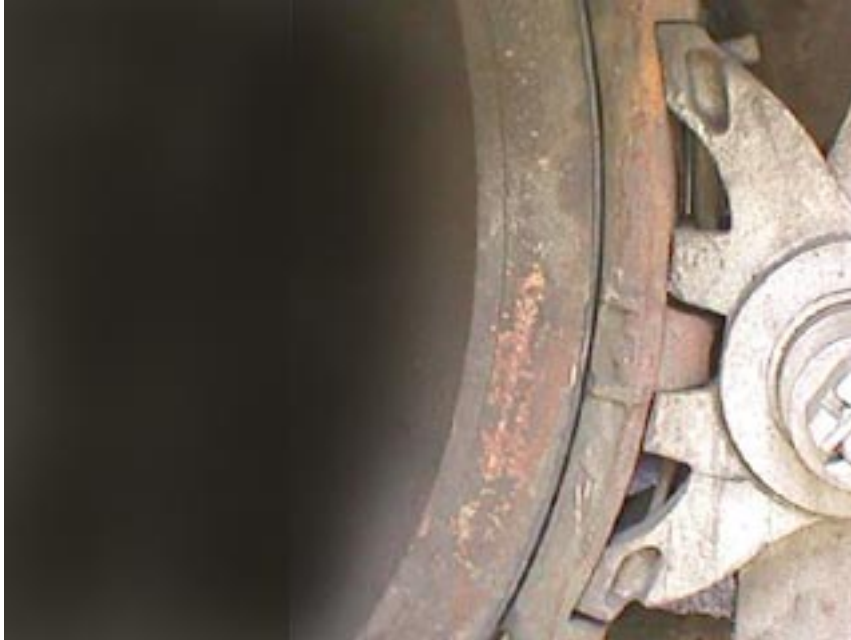
Photograph 6-4. Cast Brake Shoes (Note Wear Indicators - Center of Shoe)
