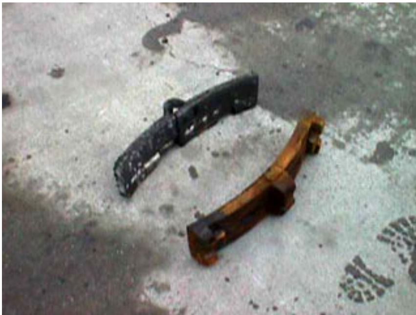
Photograph 6-5. Worn Brake Shoes (Left: Composition Shoe; Right: Cast Iron)
