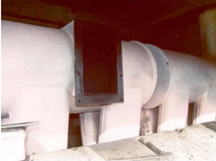
Photograph 5-6. Exhaust Clean-Out Trap on Non-Turbo Engine
