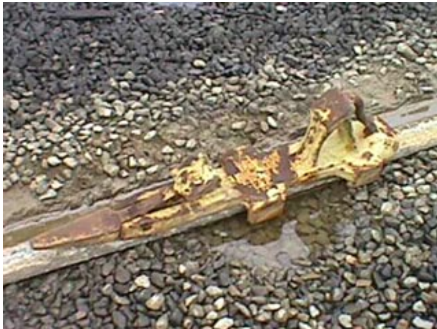
Photograph 4-3. Chock Block Device (used when train is parked)
