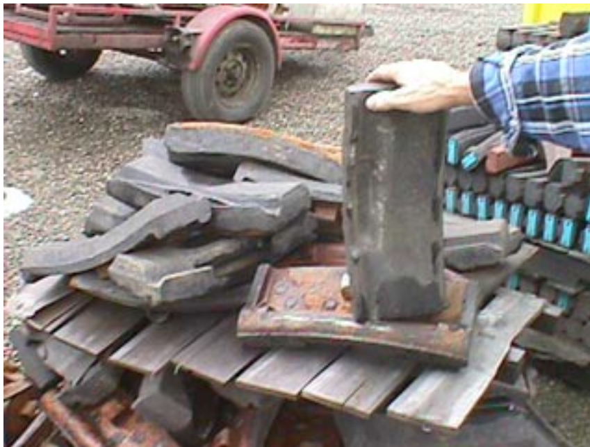
Photograph 6-3. Switch Engine, Flanged Cast Shoes (has more braking power)
