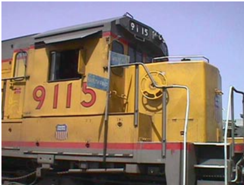
Photograph 4-1. Blue Flag (No Operation of Train while Displayed)
