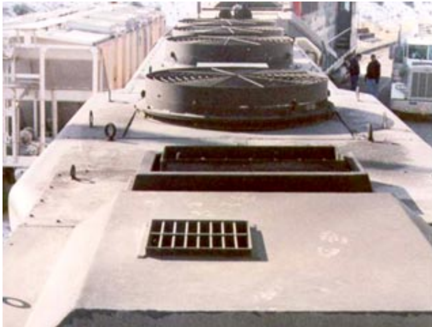
Photograph 5-15. Top of Locomotive, Exhaust Stack
