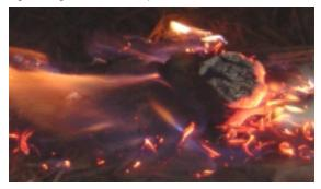
Fig. 4 Transition to flaming combustion in dried shredded hardwood mulch bed. Four ( $d_0 = 50 \text{ mm}$ ) glowing firebrand were deposited.
