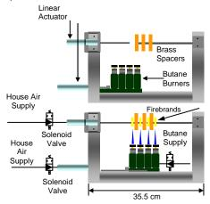
Fig. 1 Schematic of the firebrand ignition and release apparatus.
