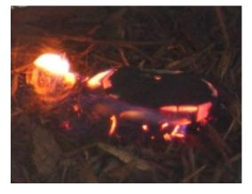
Fig. 3 Single flaming firebrand which produced flaming ignition in dried shredded hardwood mulch bed,  $d_0 = 50$  mm.
